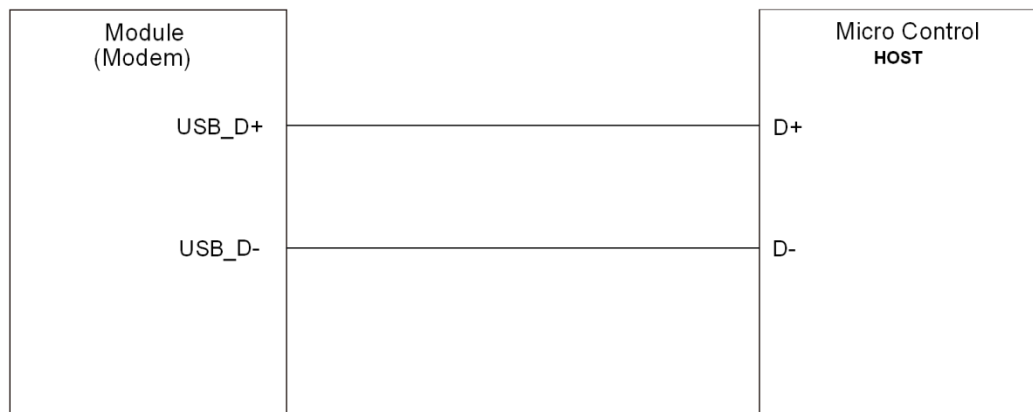
Figure 3-20 Recommended circuit of USB interface
